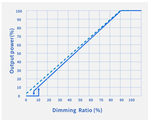
O/P Power Vs. Dimming
