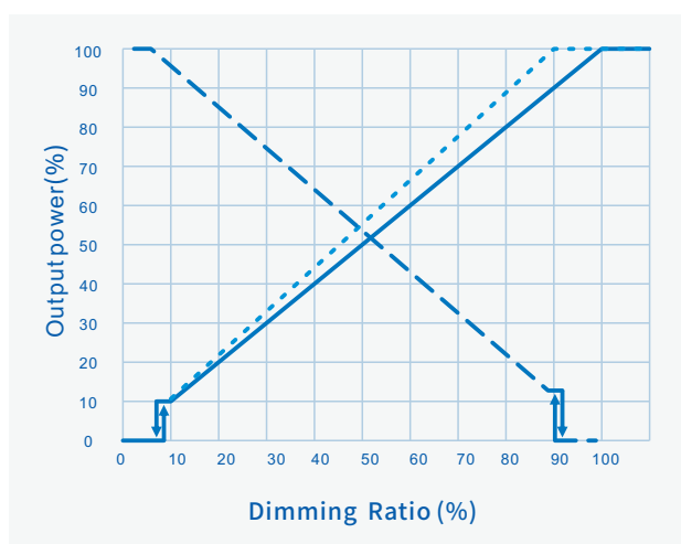
O/P Power Vs. Dimming
